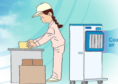
RKF never emits exhaust heat unlike an air conditioner because RKF is not equipped with a compressor.
